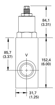
The MCV2-20 is a dual inline housing type motion control or load holding valve. This valve controls a moving load and prevents loads from running ahead of a pump. It will also lock or hold a load in any position and provides for thermal expansion relief.
