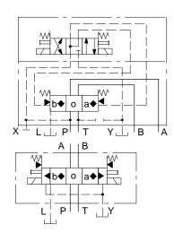
Spring Offset, End-to-Center, **Opposite Hand** Spool types Models DG5V-7-\*B 4, 8 DG5V-7-\***BL** 0, 2, 52, 521, X2▲, Y2▲
