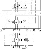
Detented, DG5V-7-\*N Spool types: 0, 2, 6, 9, 52, 521, X2▲, Y2▲
