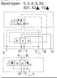
Spring Offset, End-to-End, **Opposite Hand, DG5V-7-\*AL** Spool types: 0, 2, 6, 9, 52, 521, X2**▲**, Y2**▲** b 0 а Х Р Т B A Y, İ, A В ∿Þ b а Р т
